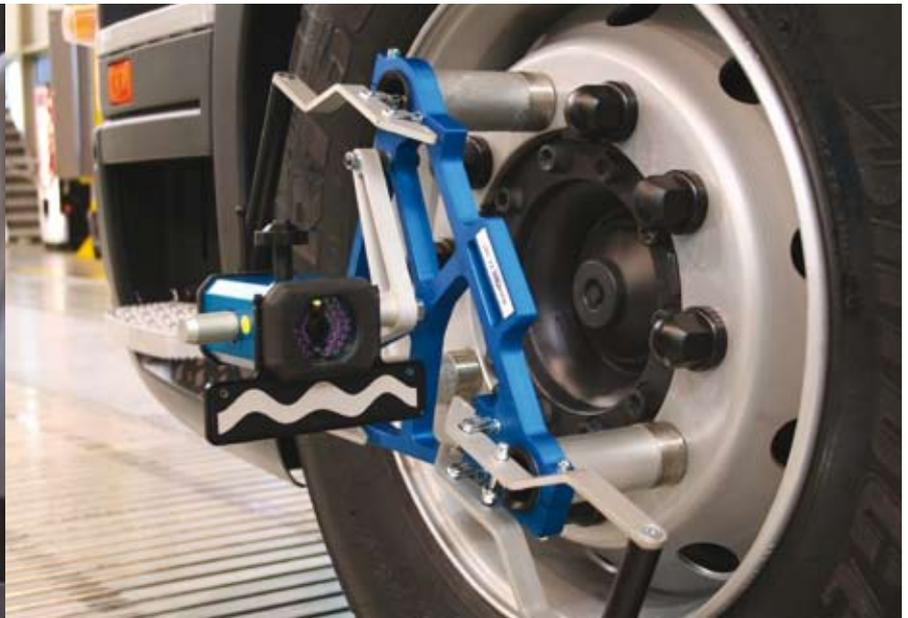
The actual measurement starts as the operator clicks the OK-button on one of the cameras, to indicate that the equipment is in place on the vehicle. The software calculates the parallelism of the front axle, using the main driven axle as the reference axle.
