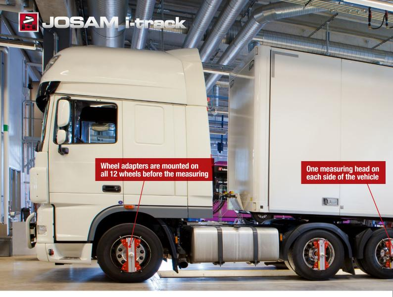
Measuring of a complete carriage (truck and semi-trailer).
