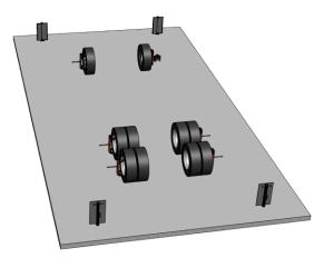
For the purpose of fast diagnostics and wheel alignment, the JOSAM i-track target scales can be mounted on a dedicated floor area with a surface up to 22 meters in length, and about 4 meters in width.
